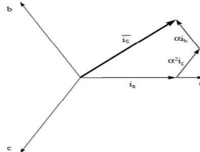
Figure14: Stator current space vector and its components in (a, b, c)
