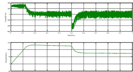
Figure 24-Variation of Step change in speed reference for actual values .
