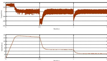
Figure 129-Variation in rotor speed and electromagnetic torque in low-speed region estimated values.
