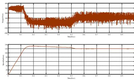
Figure 27-Variation in rotor speed and electromagnetic torque with step rise in load for estimated values.
