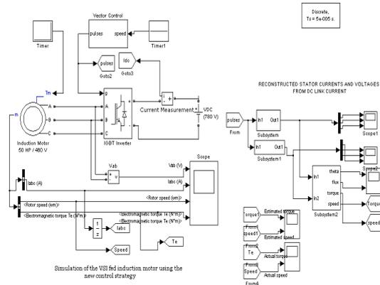
Figure 10-Simulink model of the VSI fed Induction motor speed control using DC link measurements Figure 11- Internal structure of control strategy.
