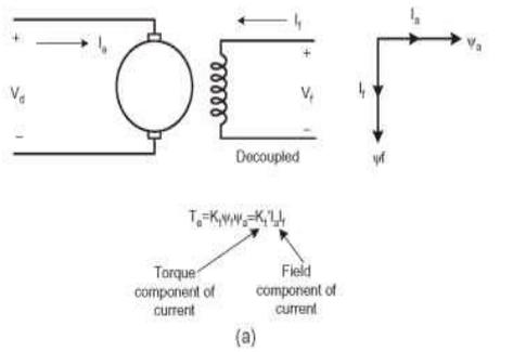
Figure12: Vector analogy of separately excited dc motor.
