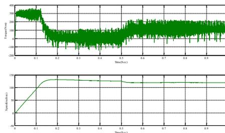
Figure 128: Variation in rotor speed and electromagnetic torque with step rise in load for actual values
