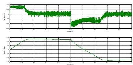
Figure126-Variation of speed reversal for actual values Step change in load-
