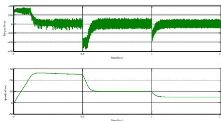
Figure 130- Variation in rotor speed and electromagnetic torque in low-speed region actual values
