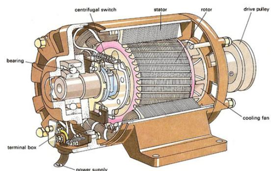
**Figure11: A simple Induction Motor.**
