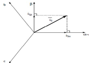
Figure 5: Stator current space vector and its components in (alpha, beta)
