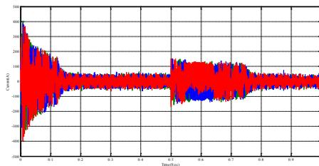
Figure 19 -Stator reconstructed currents during speed at no load reversal.
