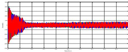
Figure117: Stator reconstructed AC line currents at rated load.
