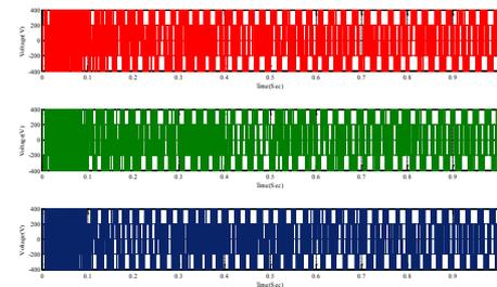
Figure 15-Reconstructed waveform of three phase voltages.
