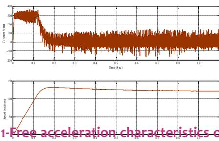
Figure121-Free acceleration characteristics of estimated torque and speed
