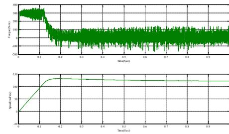
Figure122-Free acceleration characteristics of actual torque and speed.
