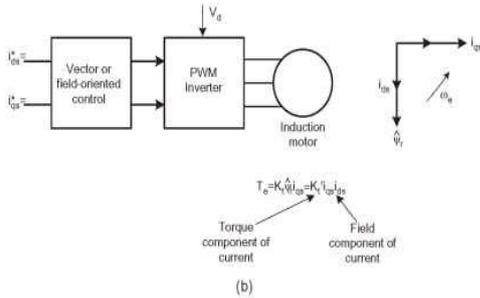
Figure13: Vector controlled induction motor.
