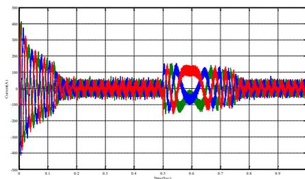
Figure 20- Stator actual currents during speed at no load reversal
