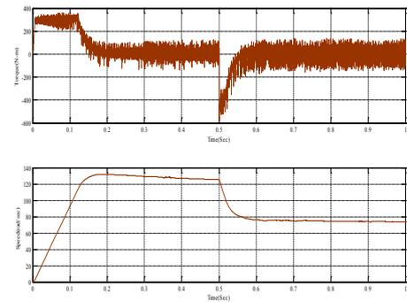
Figure123- Variation of Step change in speed reference for estimated values.
