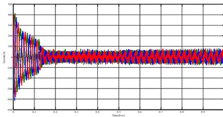
Figure118: Stator actual AC line currents at rated load.
