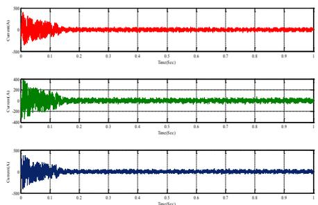
Figure16-Reconstructed waveform of three line currents
